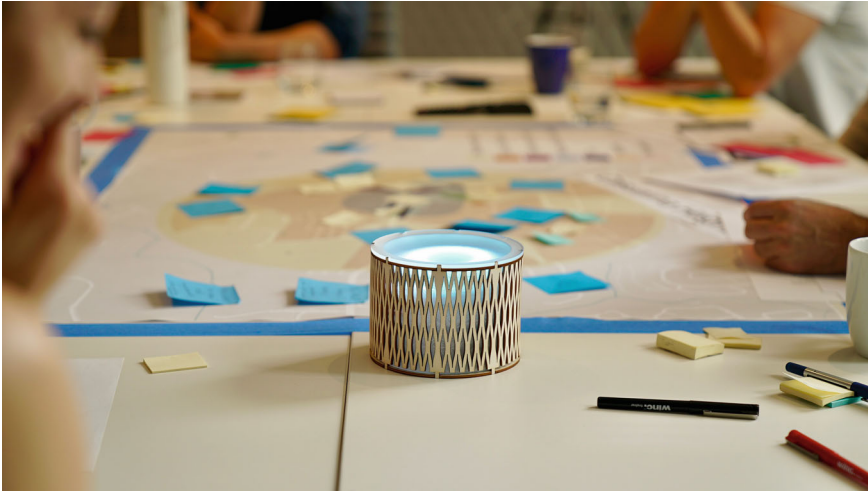
Fig. 8.1 Prototype of the conversational agent 'Sage,' represented through a custom-made device and enacted by a professional voice actor to simulate interactions in a community engagement workshop in which participants had to debate whether to rebuild or relocate their community after a major flooding event. Source Authors
